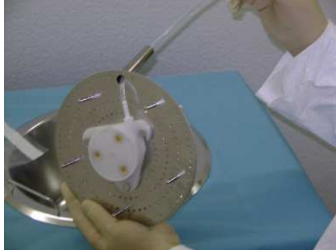
Fig. 20: no torsion on silicone tube
